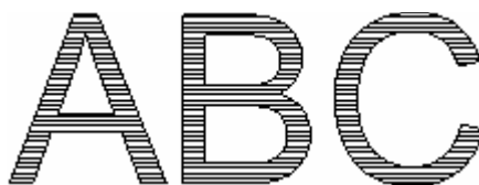
Fill spacing = 30 bits
