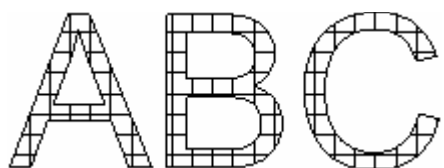
Crosshatch with 0 and 90 degrees
