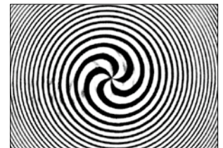
Chrome ablation for beam shaping
