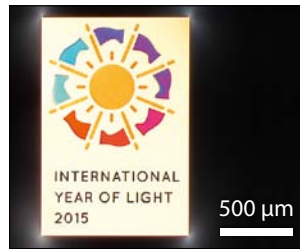
Birefringence modification inside fused silica. Photo in crossed polarized light
