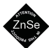
The CO<sub>2</sub> beam coupler is equipped with an optical component made of ZnSe.
