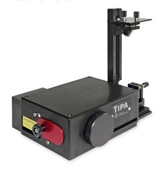
takes place. SH beam's width and tilt in a plane perpendicular to propagation provide information about the pulse duration and pulse front tilt.
